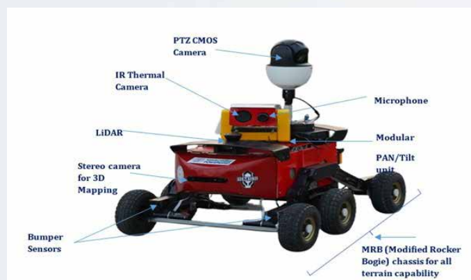
Figure 4: Robot for automated substation inspections
